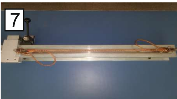
Dropper Length Verification
